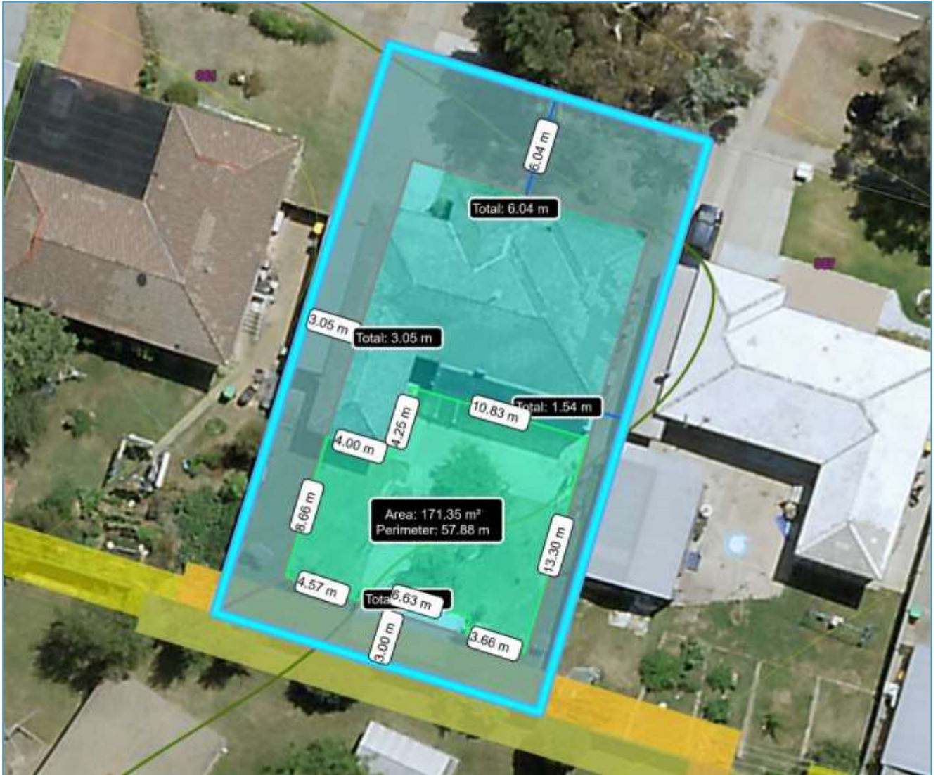
Aerial View of the Project Block with Building Offsets and Building Zone
