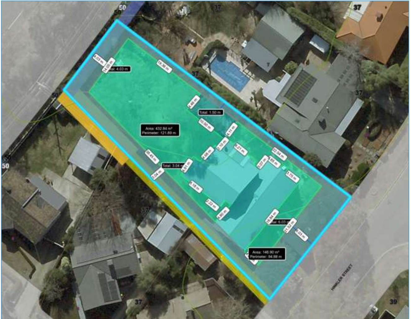
Aerial View of the Project Block with Building Offsets and Building Zone
